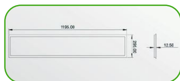
Diagram of 36W 1200x300 LED Panel
